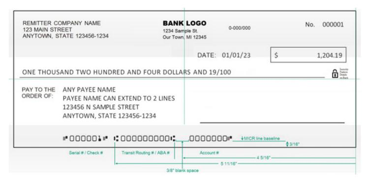
Note: Sample is not to scale. The dashed lines indicate horizontal and vertical midpoints and the right edge of the check layout.
